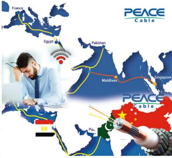
Through the deployment of the PEACE submarine cable system, Pakistan will have access to high-speed, large-volume internet bandwidth with express connectivity to France. With its ultra-low latency design, this cable will reduce latency between Pakistan and France to 92 milliseconds
